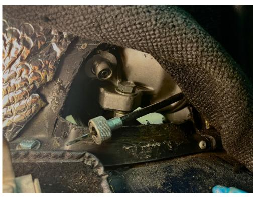
Without an access panel on a TR4A both seats and center console need to be removed with choke and heater controls. Disconnect the OD wiring, remove carpet and tunnel...then reassemble everything.
