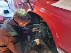
With the help of some parts and advice from Jeff Kussard, and a lot of YouTube, we got the rolling part fixed before the tech session by refurbishing or replacing most of the braking system including the master cylinder, booster, front calipers and rotors, rear drum cylinder and pads, handbrake, and a few brake lines.
