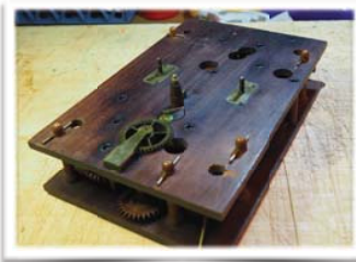
Showing the complete movement with walnut face plates. Note the sparse use of brass.
