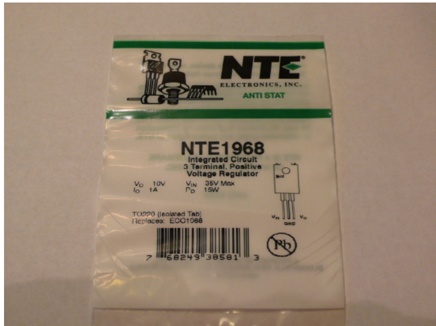
Above: The part details of the regulator: Model NTE1968. Radio Shack part # 55052569. +10 volts output at up to 1.5 amps. TO-220 case with 3 electrical "legs" for connections.
