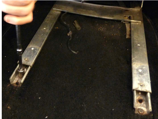
Removing back bolts. ↑ Also note there are two holes in each rail. The outboard rail uses the front hole, the inboard rail uses the back hole. Don't ask me why.
