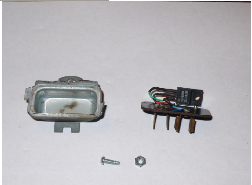
Right: The case, modified circuit board and the 4-40 screw that will mount the regulator to the side of the case
