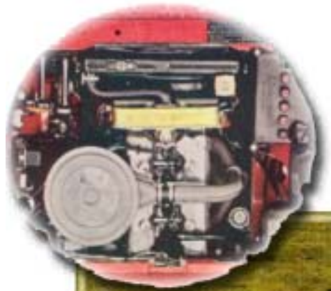
Two of the Fiat's technological tours de force: on the left is the dual overhead cam engine and below is the easily removed soft-top.
